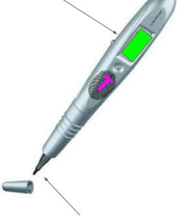
Nanoparticles on disposable tip (acting as chemoreceptors)
